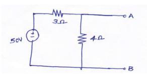
3 (a).State Nor tons theorem(b) Find Nortons equivalent circuit across AB for the circuit shown in below.
