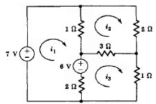
5 Find the current delivered by the source for the circuit shown in figure. 12M
